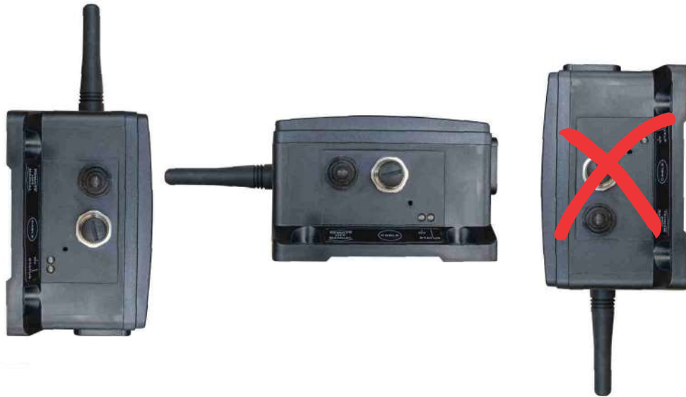
Figure 5.2 How to mount the Central Unit.
