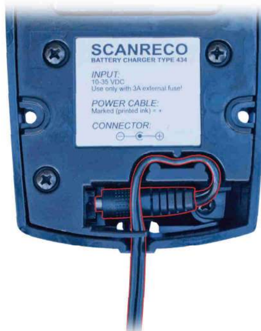
Figure 3.13 After connecting the cable connector; put the cable inside the cable track.
